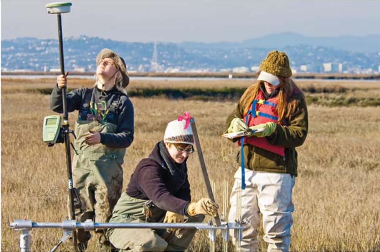
Measuring sediment deposition and elevation changes in the South Bay (at Greco Island) in 2009. About 35 millimeters of sediment had accumulated since 2000, keeping pace with sea level rise. Photo: Judy Irving, Pelican Media
